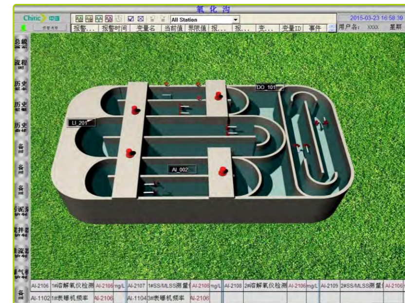
Control Chart of DO (Dissolved Oxygen) in Oxidation Ditch
